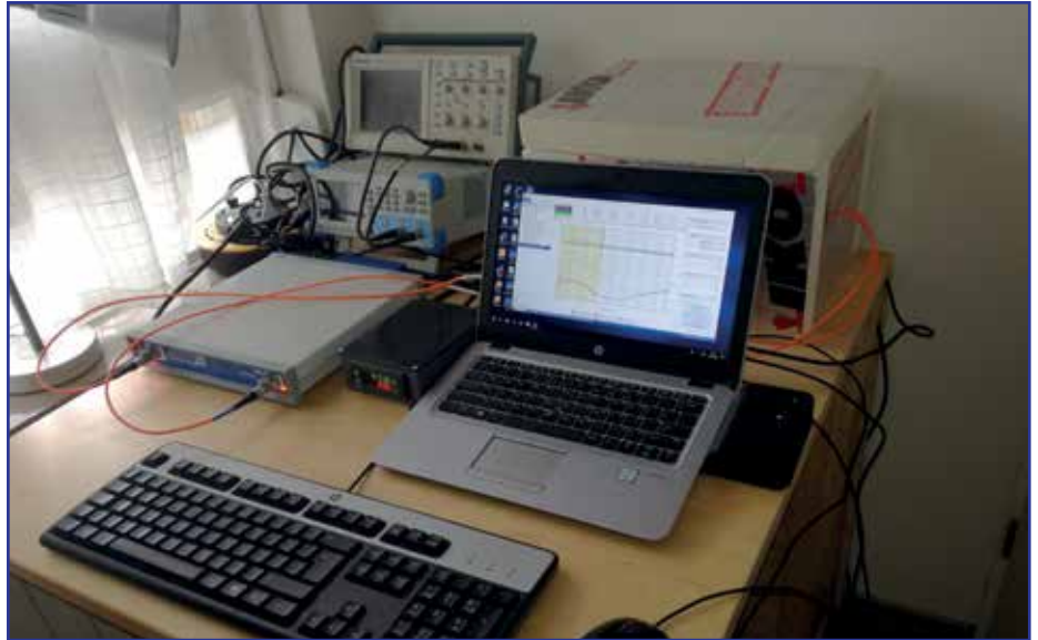
Picture 1: Dielectric study set-up
