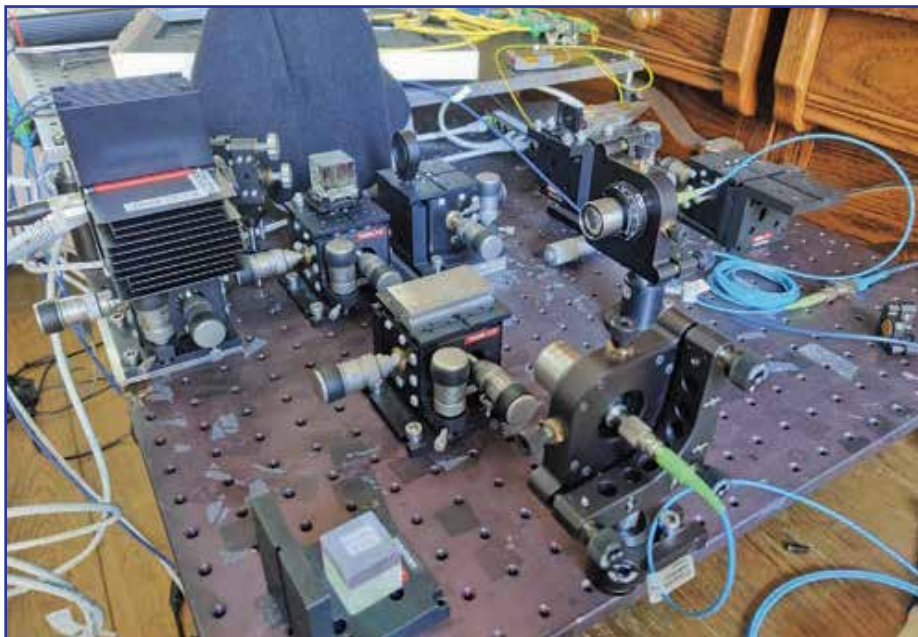
Picture 4: The portable OVNA rack with laser, photodetectors and interferometry for the fiber analysis.
