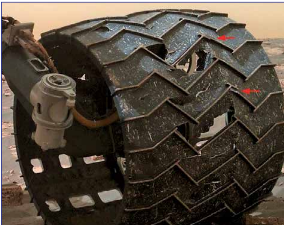
Figure 4: Collective damage on the rover's wheel during the last couple of years.
