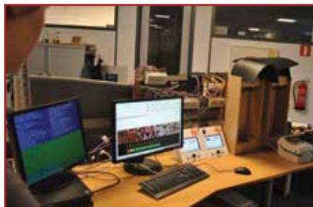
Experimental set-up to sort fruit and vegetables by visual inspection.
