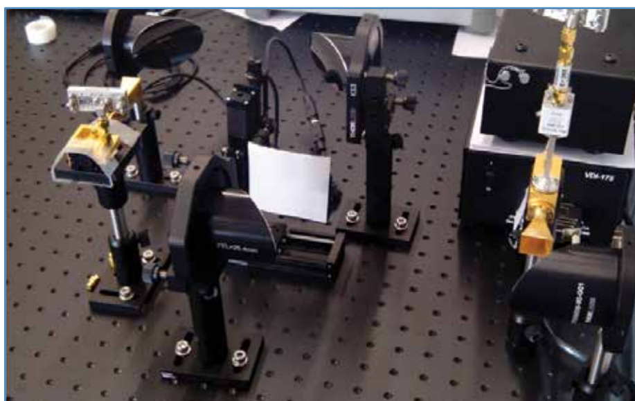
Free-space spectroscopy setup for the frequency range between 80 GHz and 120 GHz.
