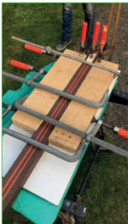
Korina body, wengé and padouk for the neck, pale moon ebony for the fretboard and ziricote for the top plate being glued together
