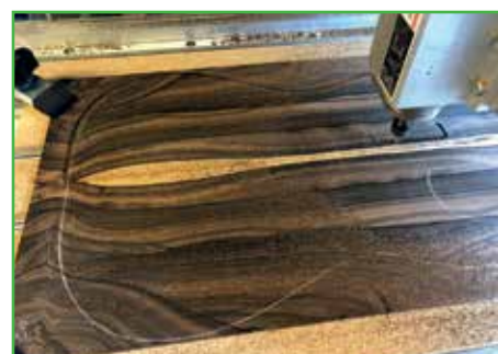
The top being machined out in the CNC machine
